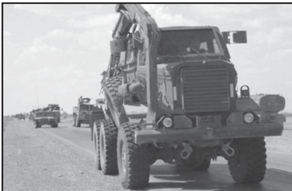
**Figure 1. Conducting route clearance in a Buffalo mine-protected vehicle**
